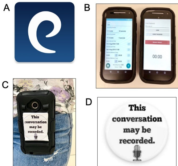
Figure 1. A) Widget image for the EAR app in the Google Play store. B) The interface that experimenters see after logging in to the EAR app (left), and what participants see once the recordings have begun (right). C) The EAR in its protective case and waist clip. D) The image printed on the bystander buttons and the stickers affixed to the phone carrying cases and armbands.
